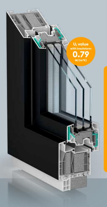
s it impossible to make PVC-U windows without steel reinforcements? While that was once the case, Kömmerling's proStratoTec technology simply replaces steel with fibreglass-reinforced plastic, which ensures a high degree of dimensional stability and rigidity.
