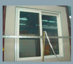
Unexposed (Inner) face of a Kömmerling PremiDoor after a BAL 40 AS 1530.8.1 Bushfire Resistance Test
