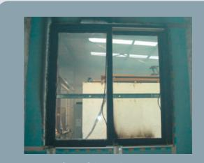
Exposed (Outer) face of a Kömmerling PremiDoor after a BAL 40 AS 1530.8.1
