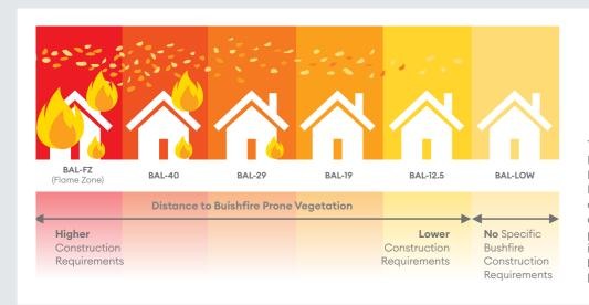
There are 6 different Bushfire Attack Levels; Low, 12.5, 19, 29, 40 and Flamezone, or FZ. These different requirements are designed to help protect both the individuals within the building and also the building itself.
