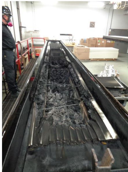
Photo No. 4 Unexposed Surface of the Test Specimen (Post-test)
